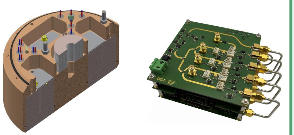
The radar uses one transmitting and three receiving antennas integrated into the melting head. In order to influence the melting process as little as possible, the antennas are made of Aluminum Nitride (AIN) ceramics offering high thermal conductivity.
