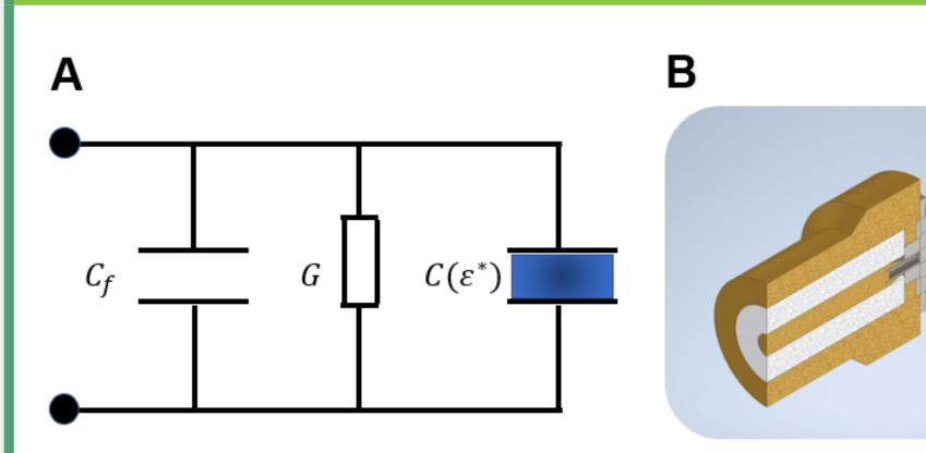
A Equivalent circuit approximation of the coaxial head: Capacitance  $C_f$ , conductivity G and variable capacitance with a dielectric of surrounding media  $C(\varepsilon_r^*)$ B CAD model of the impedance-matched coaxial head with dielectric (Teflon) filling used in the integrated FRS-system.
