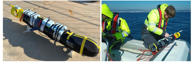
Figure 4. Breadboard model tests with Beluga nose, navigation sensors, and first OBC prototype. The Beluga nose is mounted on a commercial ecoSUB \mu 5 AUV.
